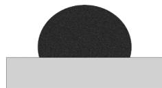
THIXOTROPIC PUR and SIL SYSTEMS To be applied onto a flat surface
