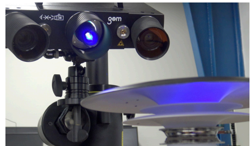
The first step is the 3D scan of our customer's lamp
