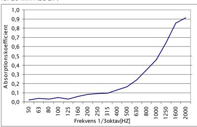
Sound absorption, A [%] according to ISO 10534-2 for 20 mm ABS 29V
